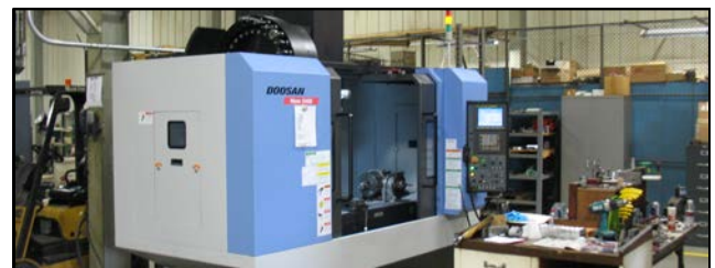
M568 DOOSAN MYNX 5400 VERTICAL M/C CENTER CAPACITY: 40"X BY 20"Y BY 21"Z
