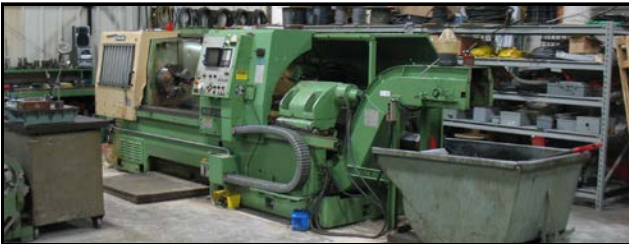
M512F MORI SEIKI TL-40 CNC TURNING CENTER CAPACITY: 18"X BY 84"Y - 24" SWING
